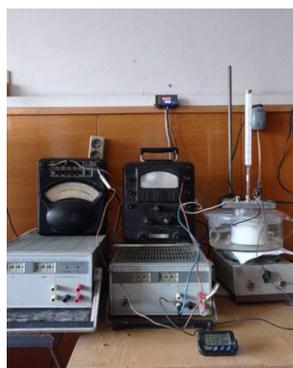
Fig. 1 – Installation for electrochemical synthesis of nanopowders
